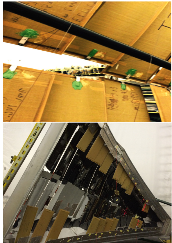
Fig. 13. Top: the gaps between mirrors before refurbishing the LTCC. These gaps were also seen in the data as a drop of efficiency near the middle of the detector, as the Cherenkov light was not collected. Bottom: all of the gaps are covered by the extension strips.
