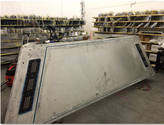
Fig. 10. View of the back-wall of the refurbished LTCC box. A stainless steel bar encapsulates a sandwich of aluminum and foam. On the left and right side of the frame, new patch panels allow for 3 hermetic connectors (1 HV, 2 signals) from each PMT.
