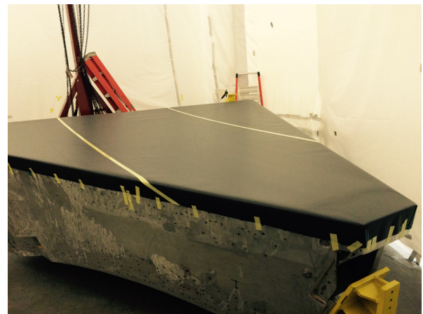
Fig. 24. The downstream window of one LTCC sector during curing of the epoxy. The two visible strips protect the window seaming.
